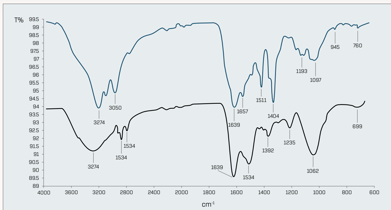
Figure 1. FTIR spectra of the Arthrospira platensis protein extract (APE) and the functionalized AuNPs-APE complex. Blue curve – the APE spectrum, and black curve – the AuNPs-APE spectrum.
